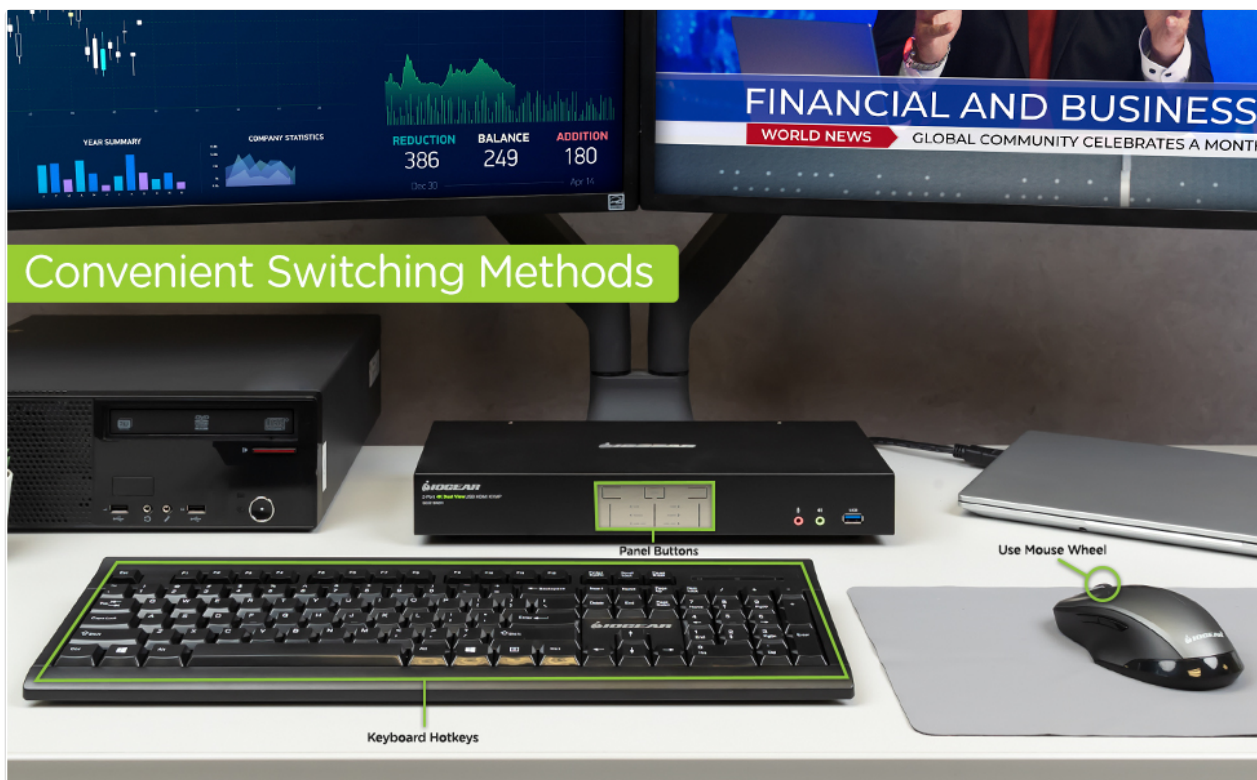
Image: A workstation illustrating the three primary methods for switching between computers: front panel buttons, keyboard hotkeys, and mouse wheel clicking.
