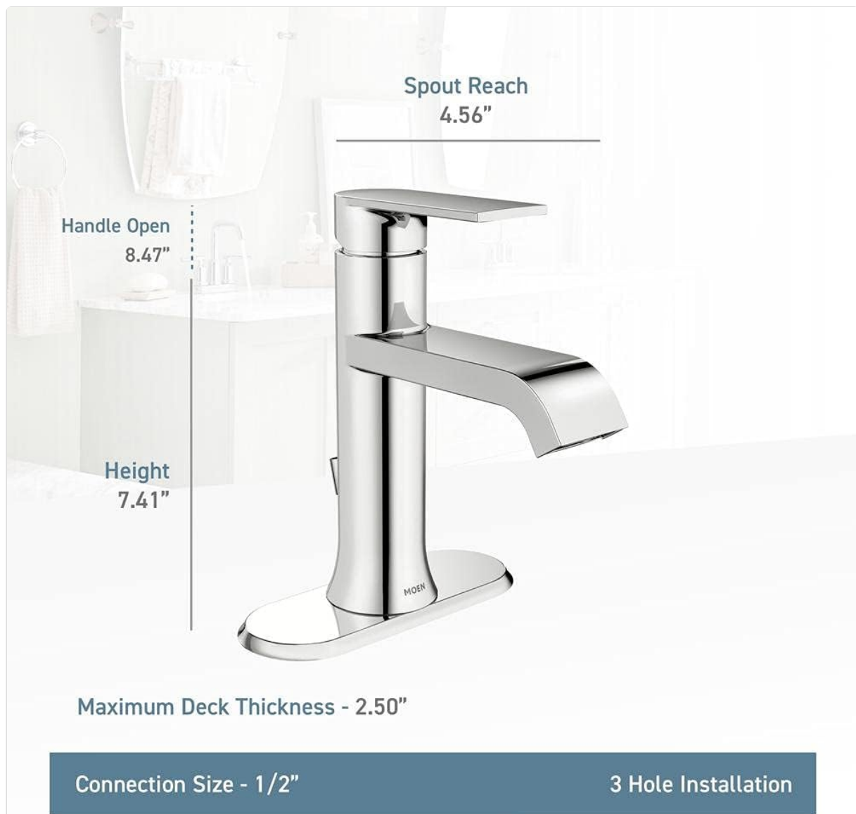
Figure 2: Faucet dimensions and installation details, including spout reach, height, and maximum deck thickness. This model supports 1-hole or 3-hole installation with the included deck plate.
