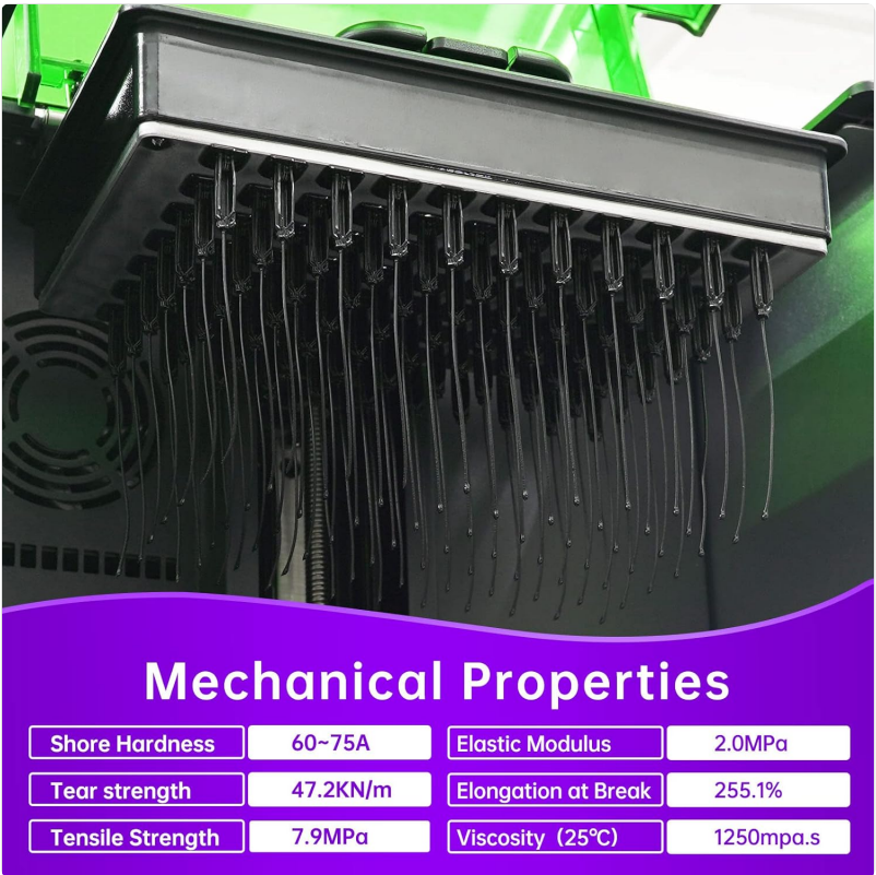
Figure 10: Detailed mechanical properties of RESIONE F69 Flexible Resin.
