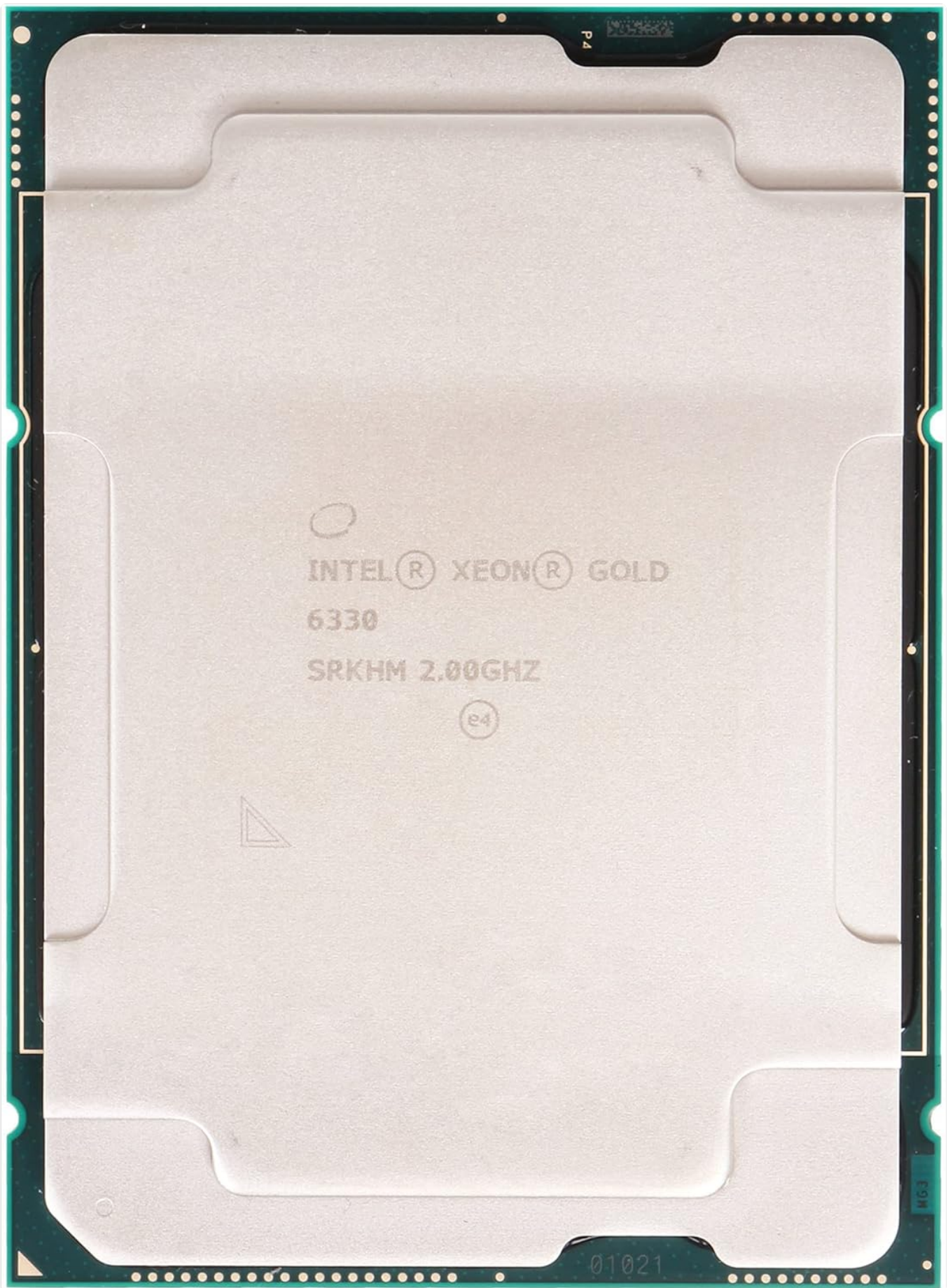
Figure 1: Top view of the Intel Xeon Gold 6330 processor, showing the integrated heat spreader (IHS) and branding. Note the alignment triangle on the corner.
