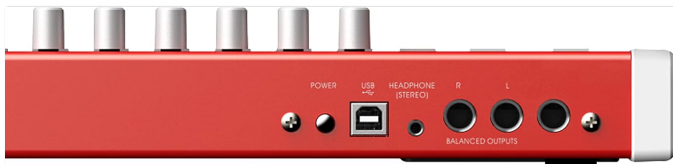
Figure 3: Rear panel of the Midiplus X6 Pro mini, highlighting the Power, USB, Headphone (Stereo), and Balanced Outputs (R, L) ports.
