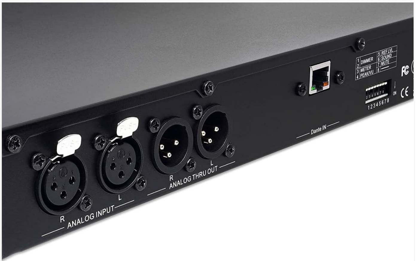
Figure 4: Close-up of the rear panel, showing the DIP switches for various settings like Dimmer, Meter type, Mute, and Peak VU.
