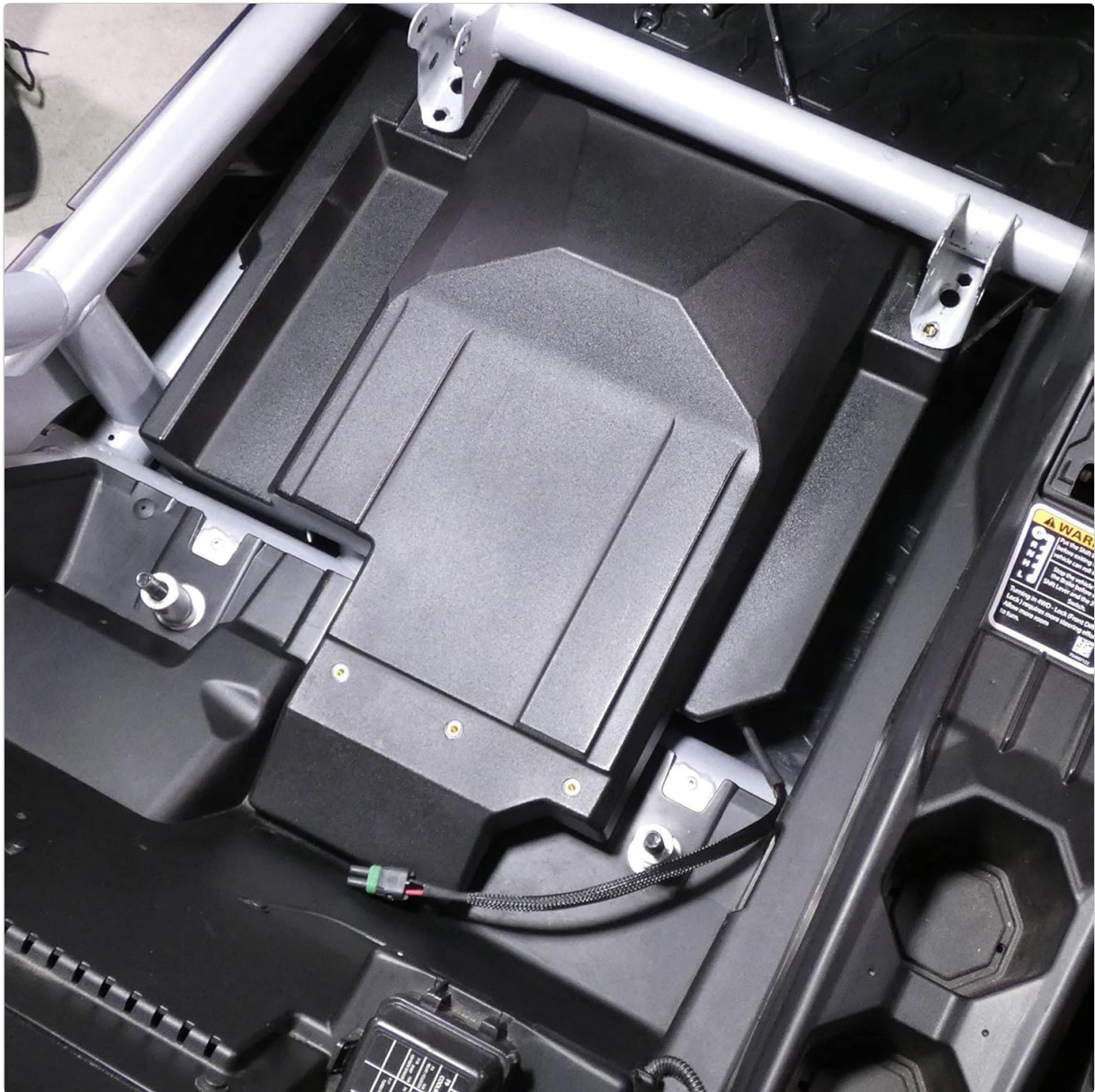
Image: The MTX Audio subwoofer enclosure shown installed under the driver's seat of a Can-Am Maverick X3. The enclosure is designed to fit snugly in the available space.
