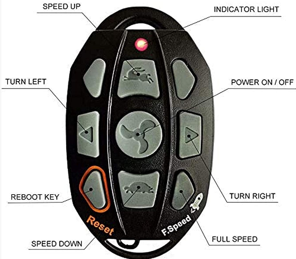
Image 5.2: Detailed diagram of the wireless remote control, indicating buttons for Power On/Off, Speed Up, Speed Down, Full Speed, Turn Left, Turn Right, Reboot Key, and Indicator Light.
