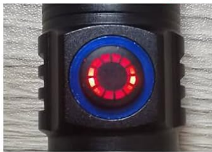
Figure 3: Charging indicator status. Red indicates charging or low battery, green indicates fully charged.
