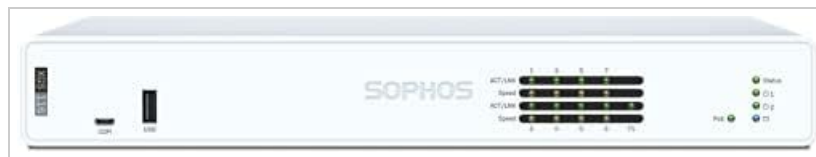
Figure 3.1: Front panel of the Sophos XGS 116, highlighting connectivity ports and status indicators.
