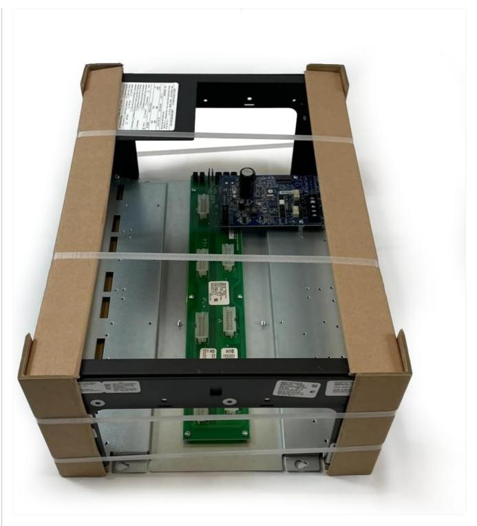
Figure 3.1: Simplex 4100-9610 Remote Annunciator as typically packaged. The image shows the annunciator unit, which consists of a metal enclosure housing circuit boards and connectors, secured within cardboard protective corners and plastic strapping.
