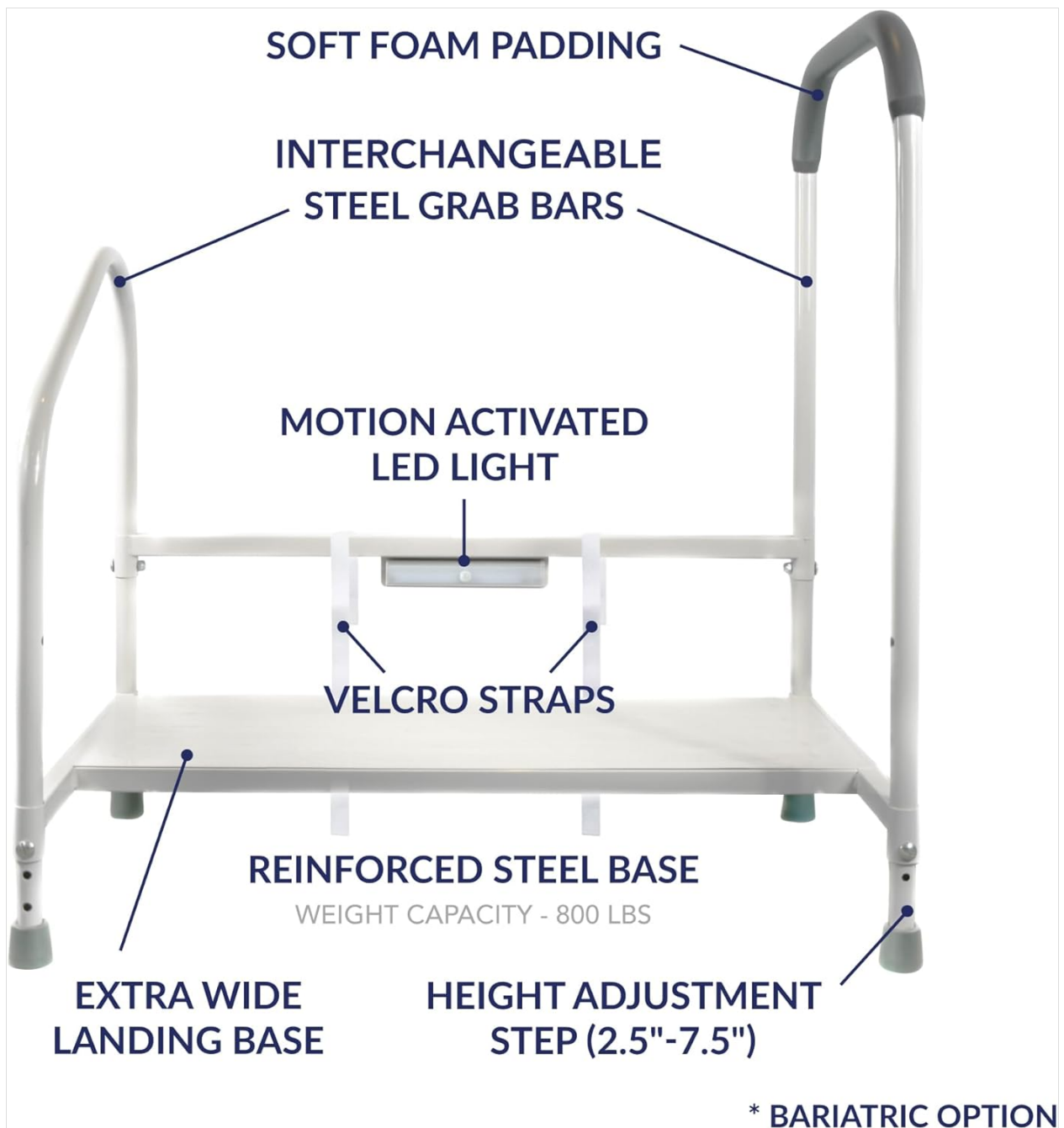
Figure 3: Key features of the step2bed XL, including soft foam padding on grab bars, motion-activated LED light, Velcro straps for securing, reinforced steel base, and height adjustment points.
