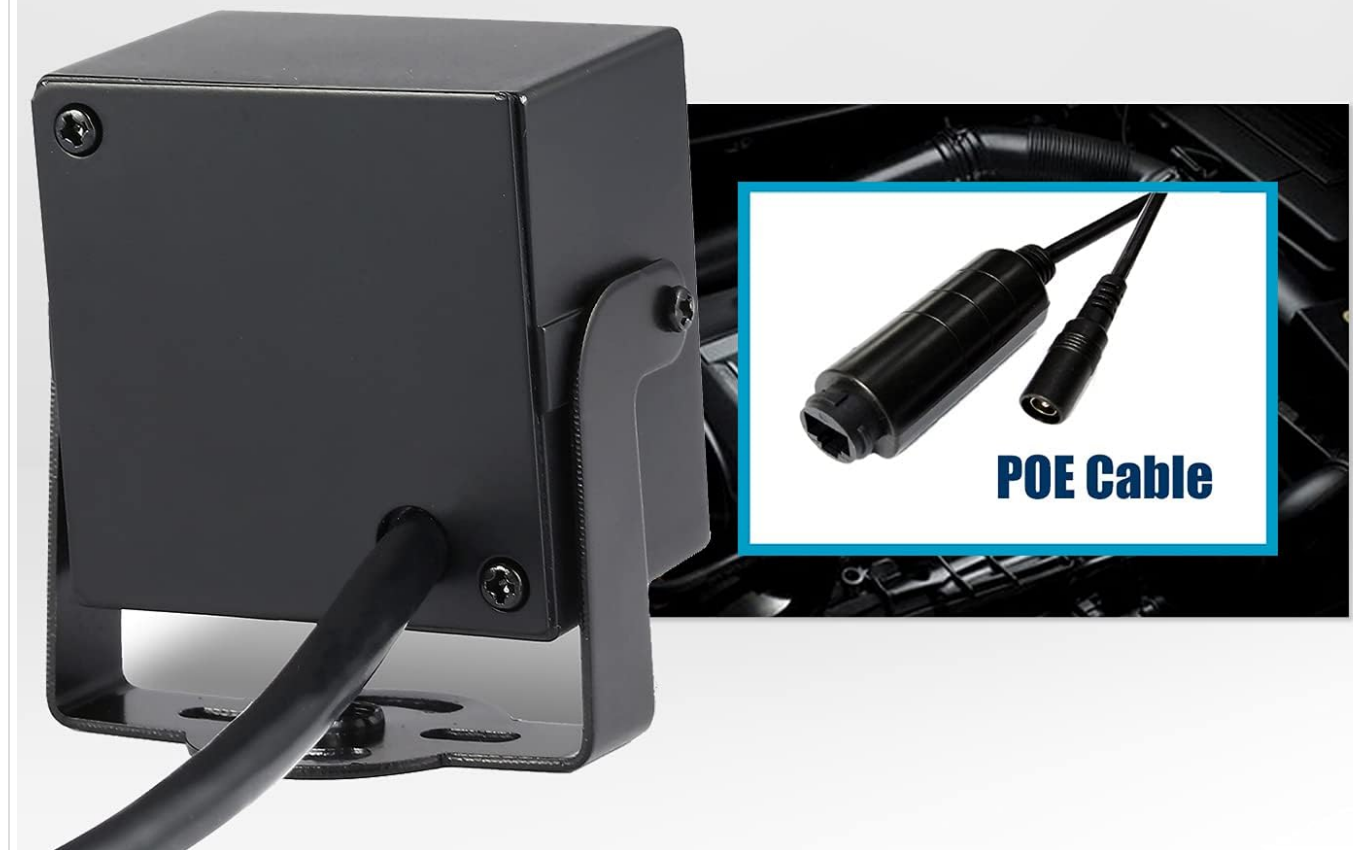
Figure 5: POE Connection Example
