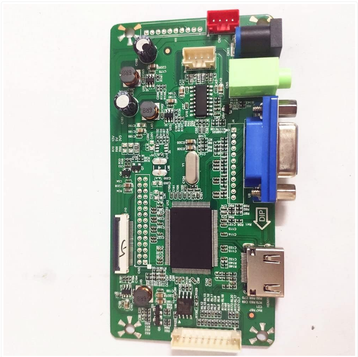
The main EDP controller driver board, featuring HDMI and VGA input ports, audio output, and various connectors for the LCD panel and control keyboard.
