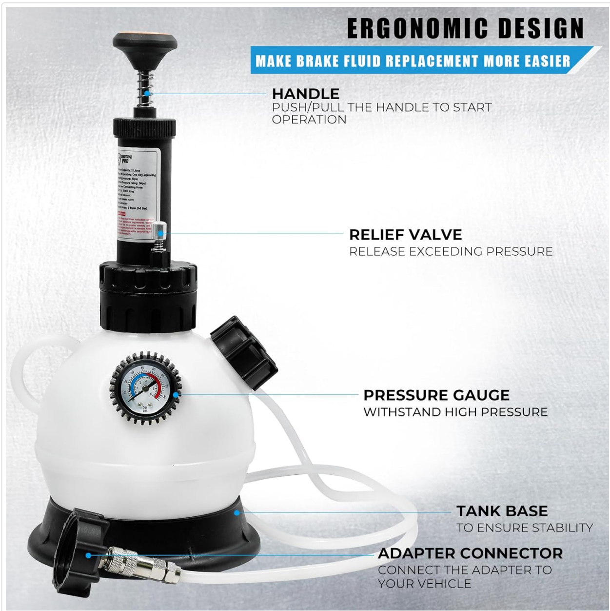
Figure 2.2: Detailed view of the brake bleeder pump highlighting the handle, relief valve, pressure gauge, tank base, and adapter connector.
