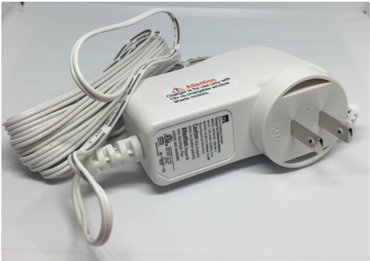
Figure 3.1: Side view of the recharger, highlighting the warning label indicating use only with 12V rechargeable window shade motors.
