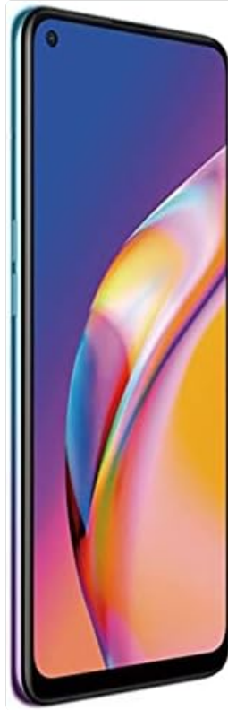
Image: Side view of the OPPO Reno5 Z 5G, highlighting its ultra-thin profile of approximately 7.8mm.
