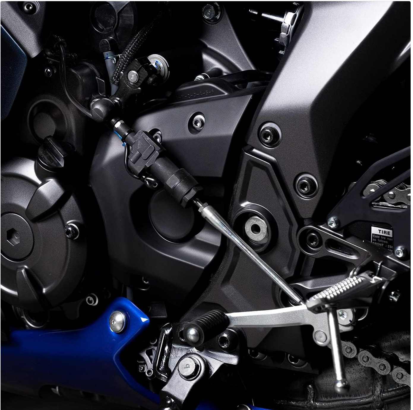
Figure 1: The Yamaha GYTR Quick Shifter Kit installed on a motorcycle engine. This image shows the quick shifter unit connected to the shift rod, positioned near the engine casing and footpeg assembly. The unit is black, contrasting with the metallic silver shift rod and blue engine cover accents.
