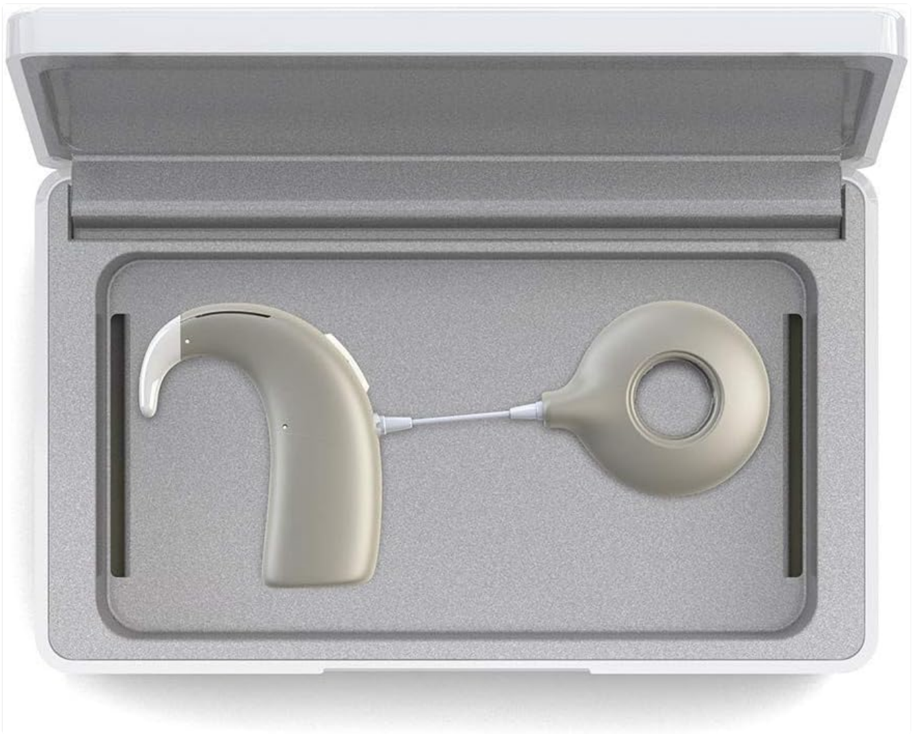
Figure 4: Placing a cochlear implant in the drying chamber.
