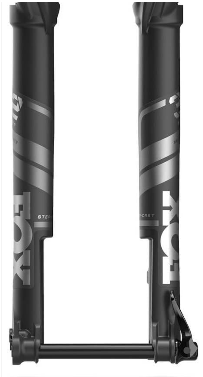
Figure 1: Front view of the FOX 32 Step-Cast Performance fork, showcasing its matte black finish and distinct Step-Cast lower leg design.
