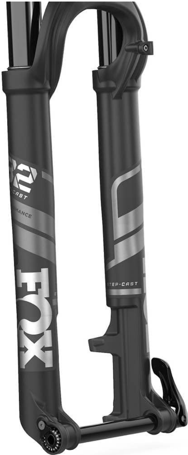
Figure 2: Angled view of the fork, illustrating the unique Step-Cast chassis which reduces weight and provides clearance for bike components.
