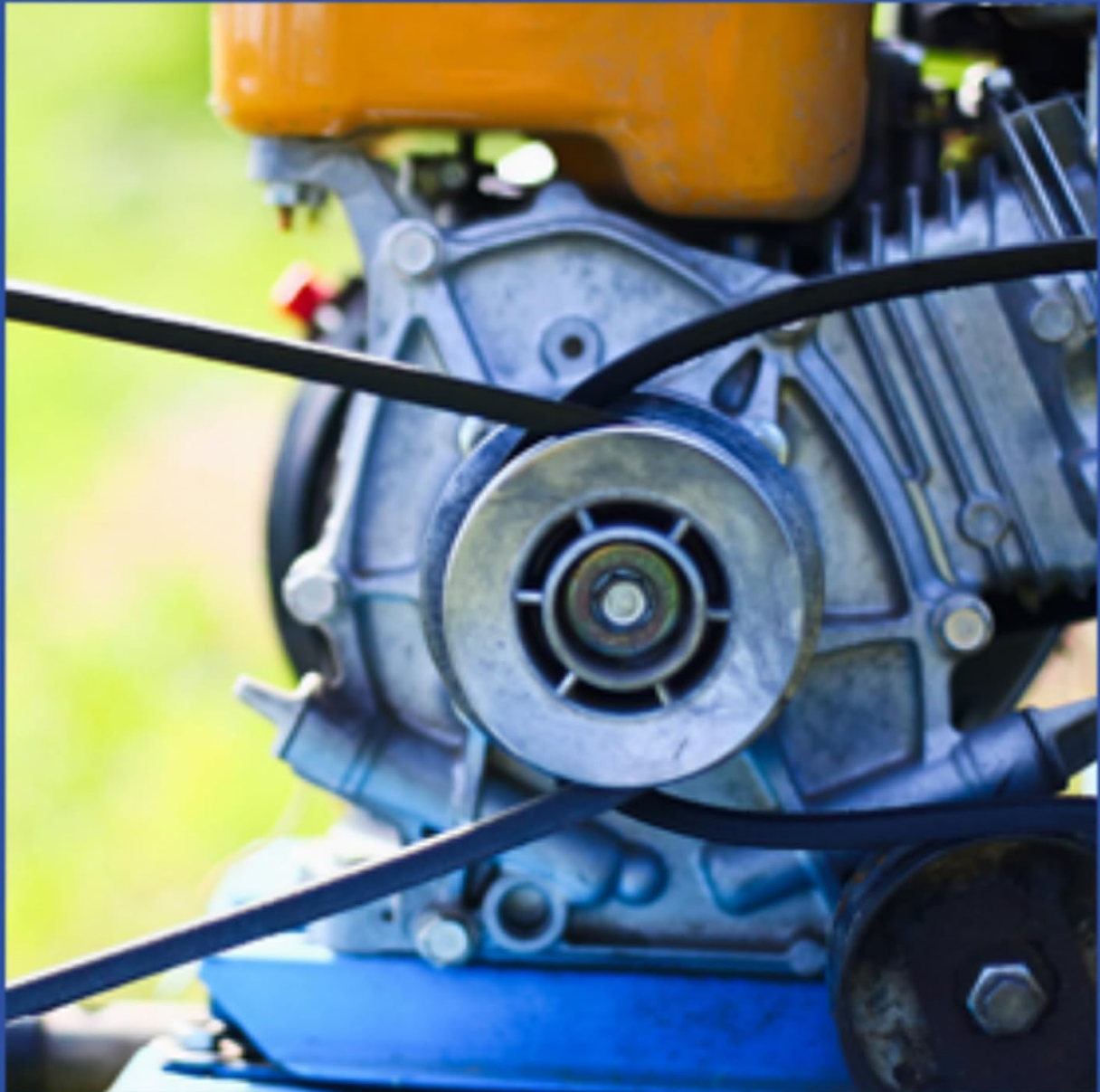
Image 5.1: A drive belt correctly seated on an engine pulley, illustrating proper routing.
