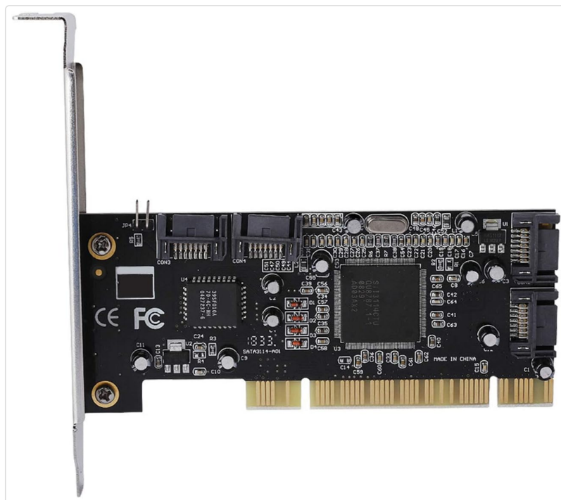
Image: Top-down view of the expansion card, highlighting the four internal SATA ports (CON1, CON2, CON3, CON4) and the PCI interface.
