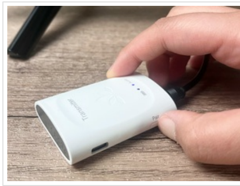
Figure 3.3: Close-up of the transmitter's pairing button, essential for establishing wireless connections with receivers.
