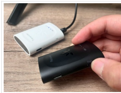
Figure 3.4: The transmitter and a receiver during the pairing process, indicated by flashing lights.
