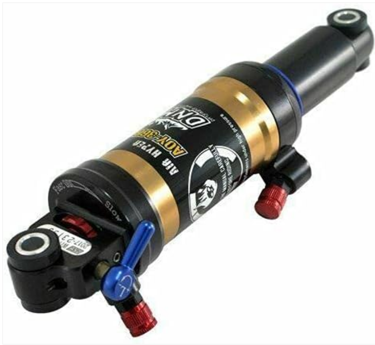
Figure 3: The DNM AOY-36RC shock with visible rebound and lockout adjusters.
