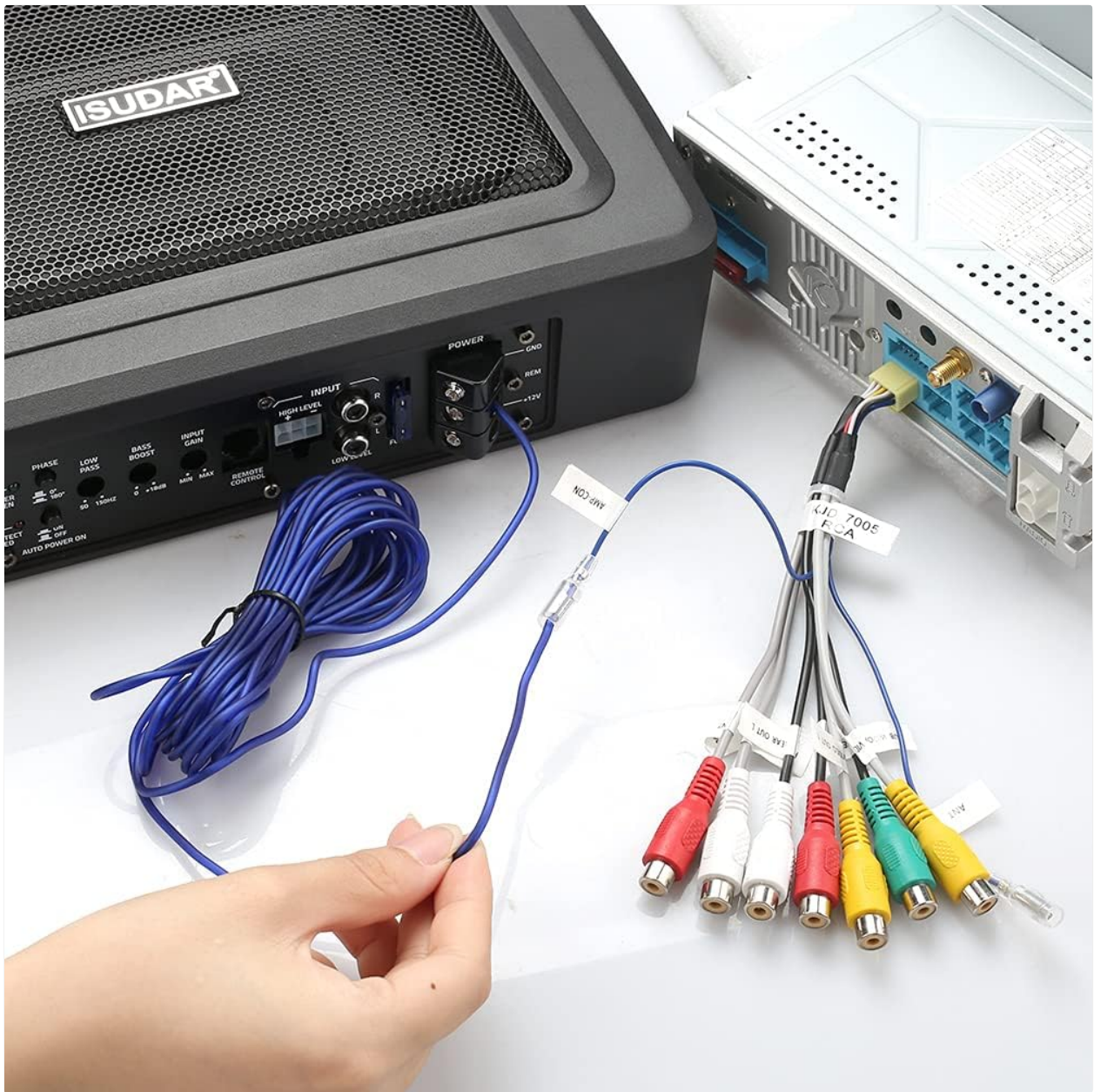
Figure 6.3: High-level speaker wire input connection.
