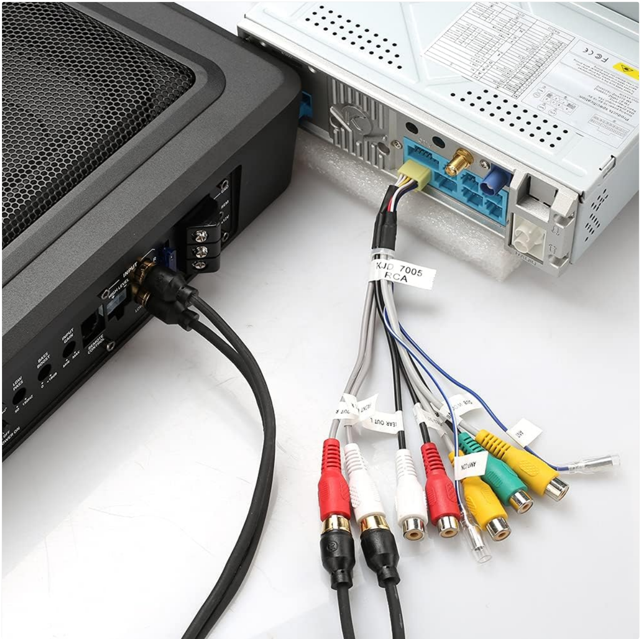
Figure 6.2: RCA audio input connection.
