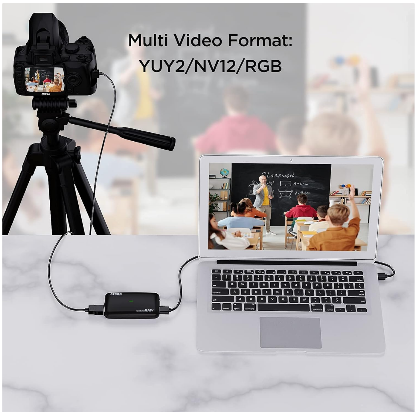
Figure 3.4: The ezcap Ezcap321 supports multiple video output formats including YUY2, NV12, and RGB, making it versatile for various video sources like DSLR cameras for educational or creative content.
