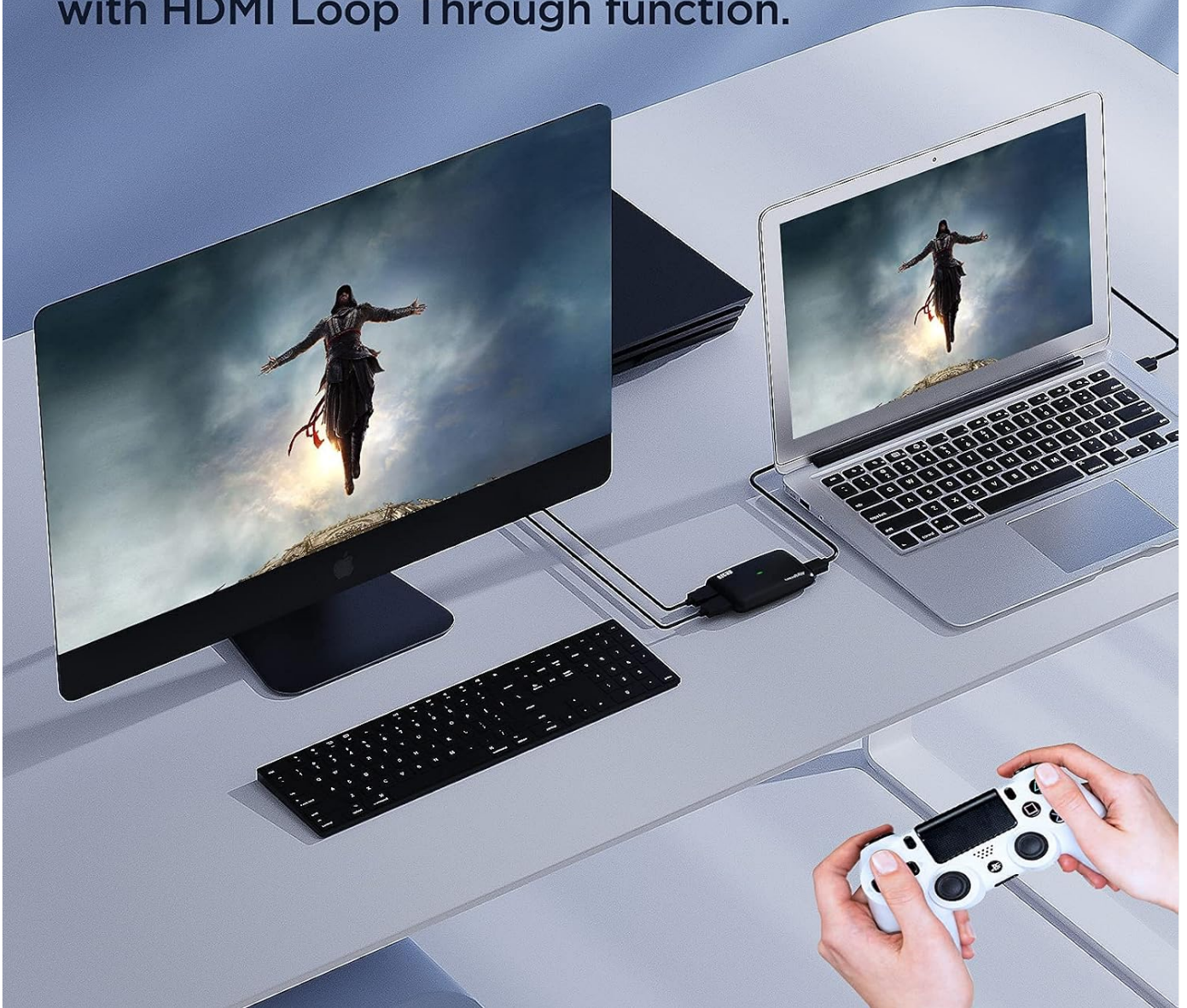
Figure 2.1: This setup shows the ezcap Ezcap321 capturing and live streaming game video from a PlayStation console. The HDMI loop-through function allows the game to be displayed on a separate monitor without delay while simultaneously being sent to the computer for capture.
