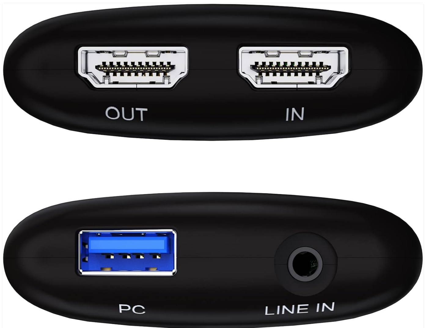
Figure 1.1: Top and bottom view of the ezcap Ezcap321 capture card showing all ports. The top side features HDMI IN and HDMI OUT ports for video signal passthrough. The bottom side includes a USB 3.1 port for connection to a computer and a 3.5mm Line In port for audio input.
