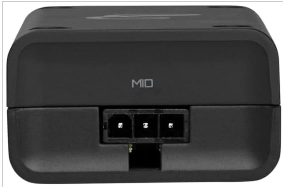
Figure 6: The KAPPA203S crossover module, indicating the midrange output connection.
