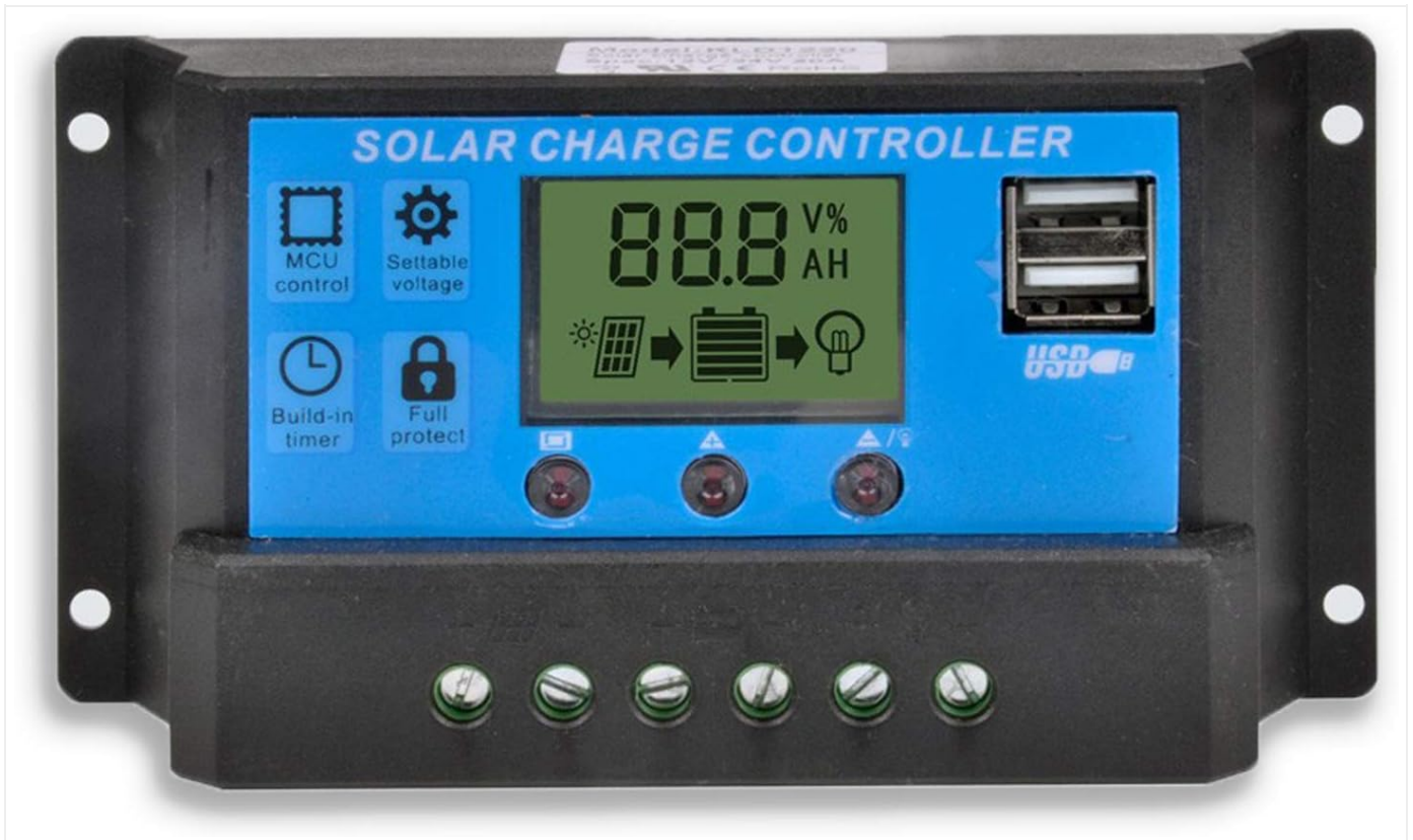
Figure 1: Front view of the Saoer 20A Solar Charge Controller.
