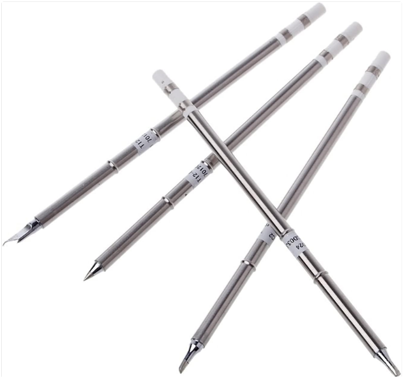
Figure 2: Full view of T12 Series Soldering Iron Tips. This image shows four soldering tips arranged in an 'X' pattern, revealing their complete length and the white ceramic heating elements at the base of each tip.
