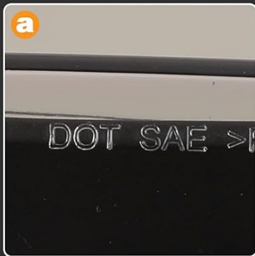
Image: Close-up view of the fog light highlighting DOT/SAE compliance markings, bulb location, and the excellent sealing around the lens.
