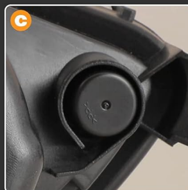
Image: Rear view of the fog light showing the light dimmer screw for adjustment, the sealing ring for bulb access, and the waterproof seal cap.
