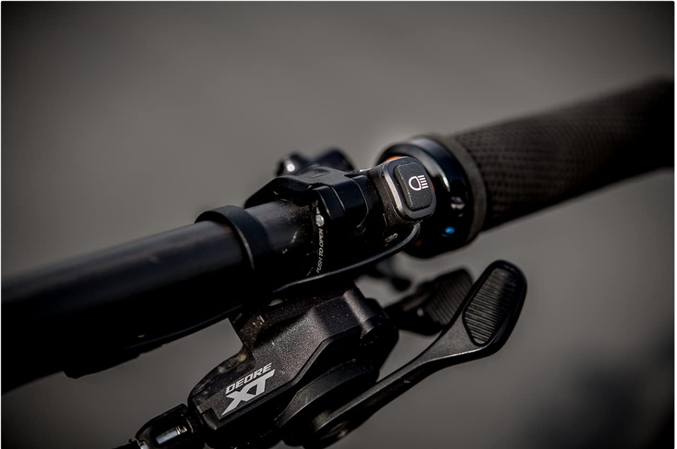
Image: Detailed view of the Litemove AE-130 control switch button, which activates the high/low beam function.
