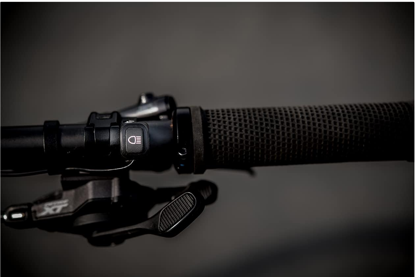
Image: Close-up of the Litemove AE-130 control switch mounted on an E-bike handlebar, showing its ergonomic placement near the grip.
