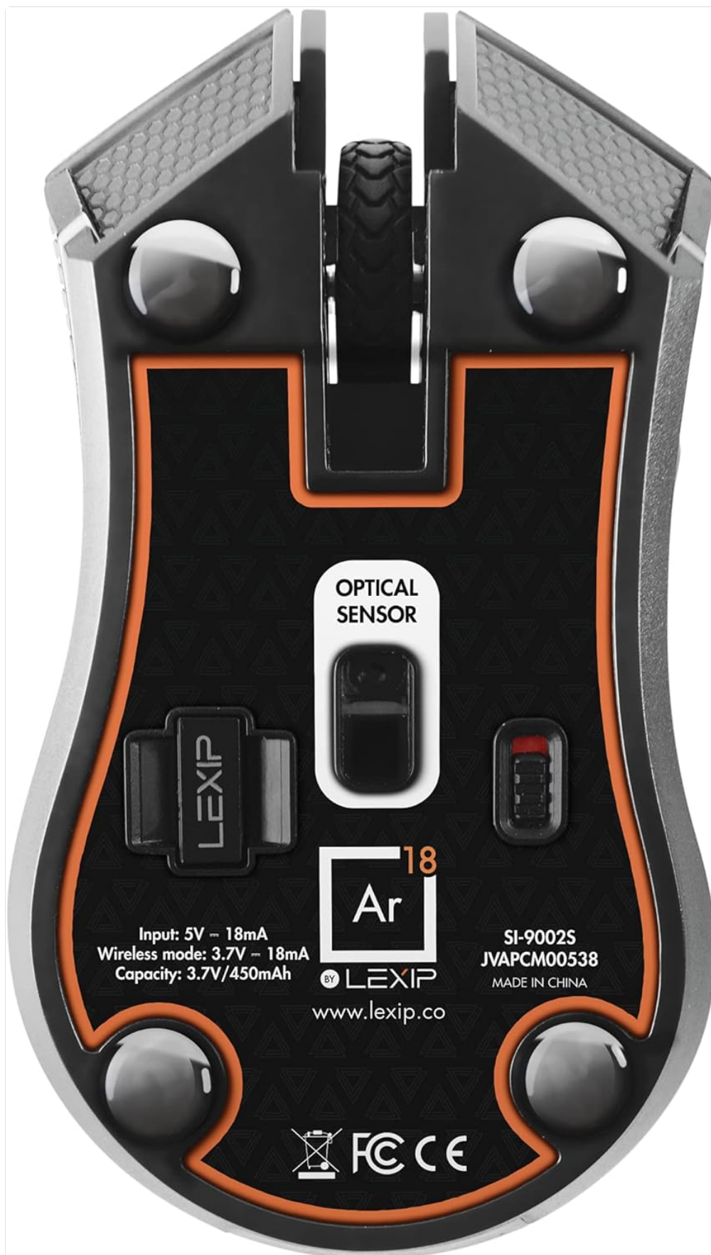
Figure 6: The underside of the Lexip Ar18 mouse, highlighting the four ceramic skates and the optical sensor.
