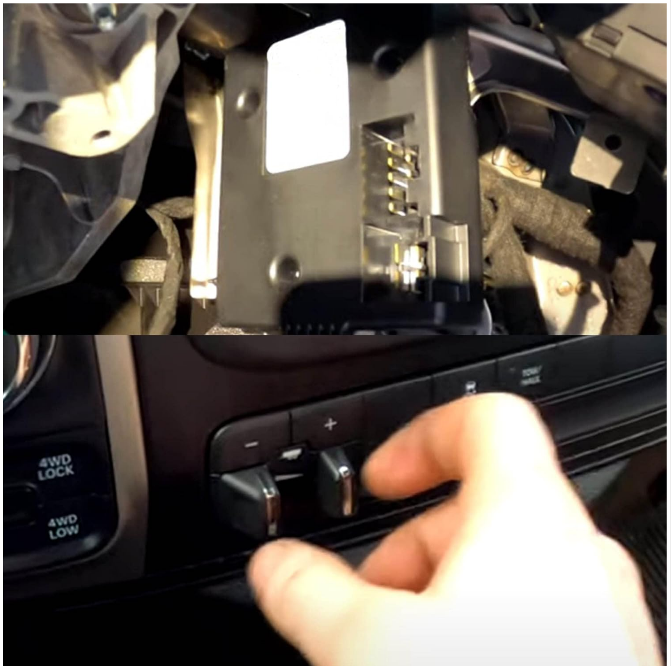
Image 6.2: A hand demonstrating the operation of the trailer brake controller switch within a vehicle's interior.
