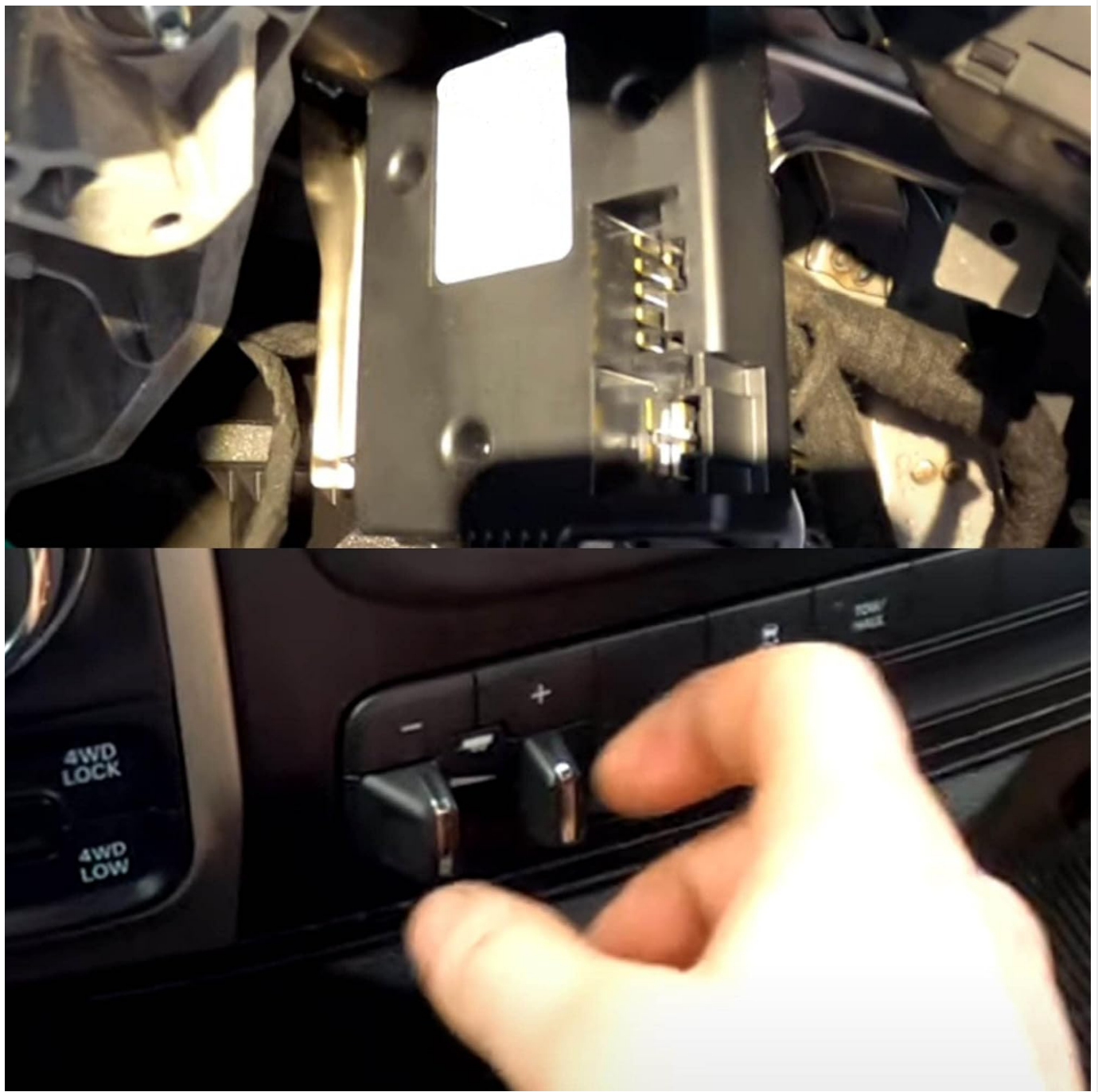
Image 5.2: Example of the trailer brake controller module installed within the vehicle's dashboard area.
