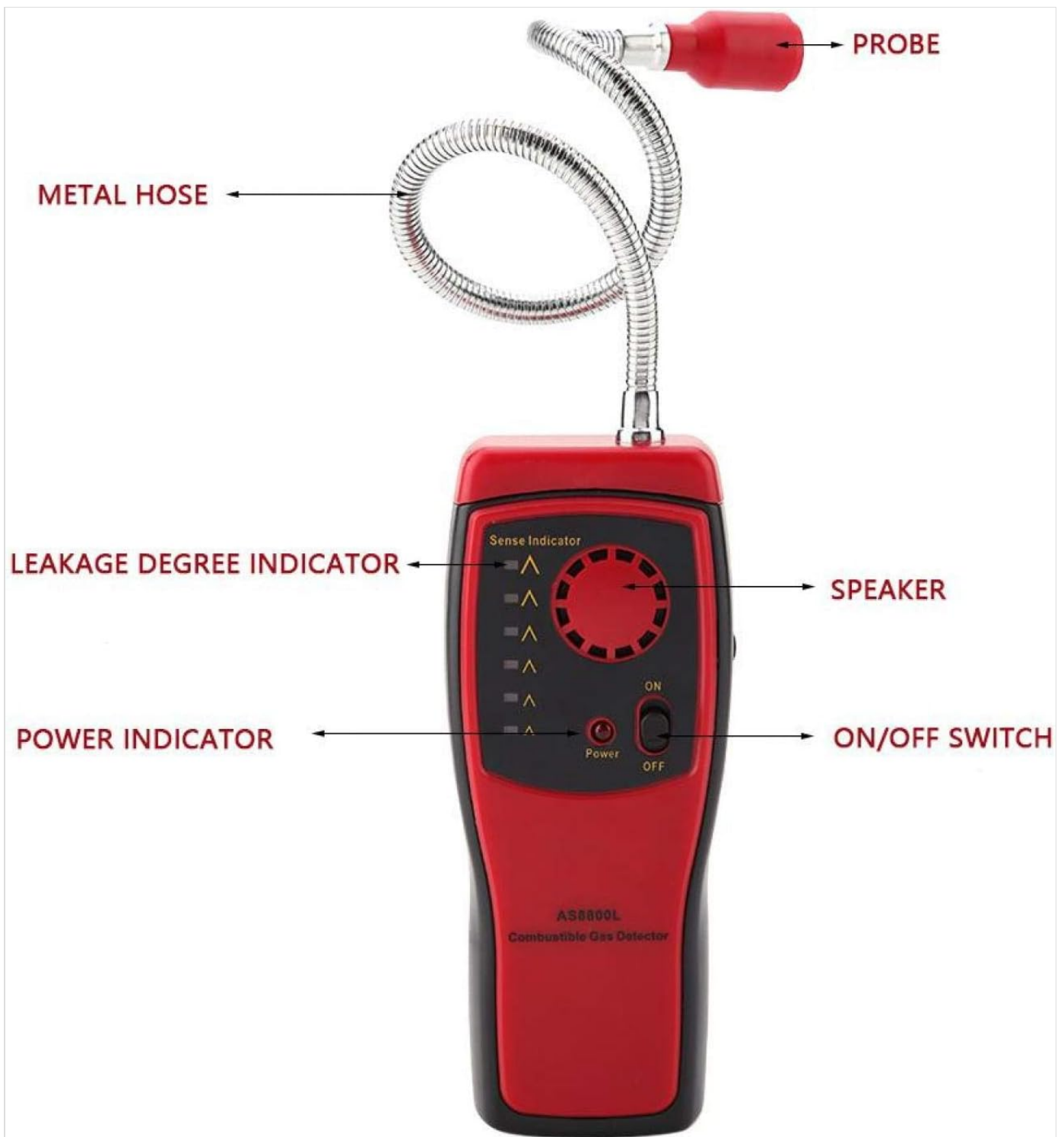
Figure 4.3: Labeled diagram of the AS8800L Gas Detector, indicating the probe, metal hose, leakage degree indicator, power indicator, speaker, and ON/OFF switch.
