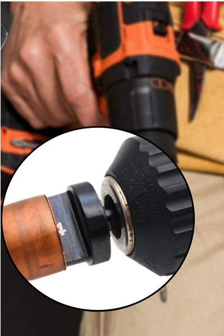
Image 5: An illustration of the swaging process, showing a copper pipe being expanded by the drill bit attached to an electric drill, alongside examples of finished swaged pipes.
