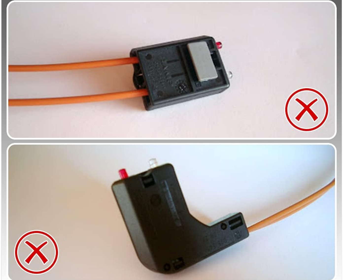
Image 2.2: Examples of D2B optical bus system connectors, which are incompatible with the MOAGW-1 decoder box. These connectors typically have a different form factor than the MOST system.
