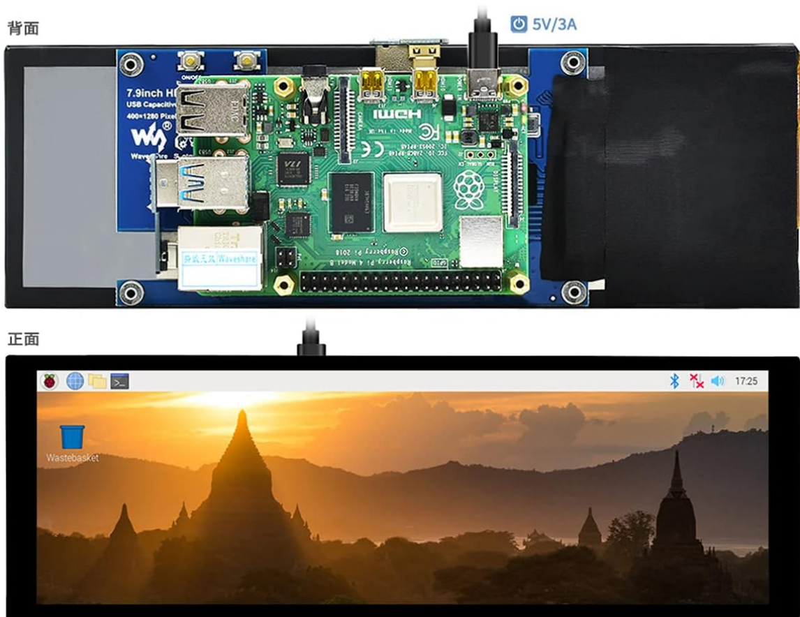
Image 3: Example of connecting the display to a Raspberry Pi 4.
