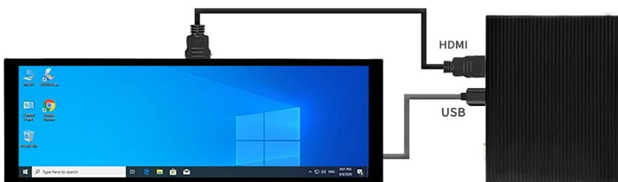
Image 2: Connection examples for Raspberry Pi Zero W, Jetson Nano, and Mini PC.
