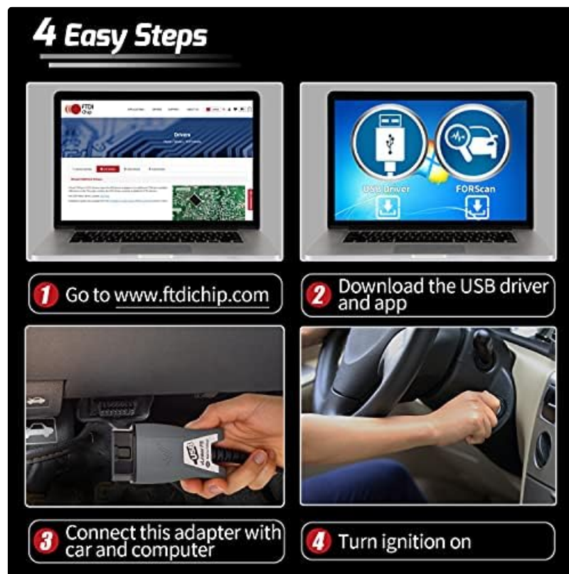
Figure 2: 4 Easy Steps for Driver and Software Installation
