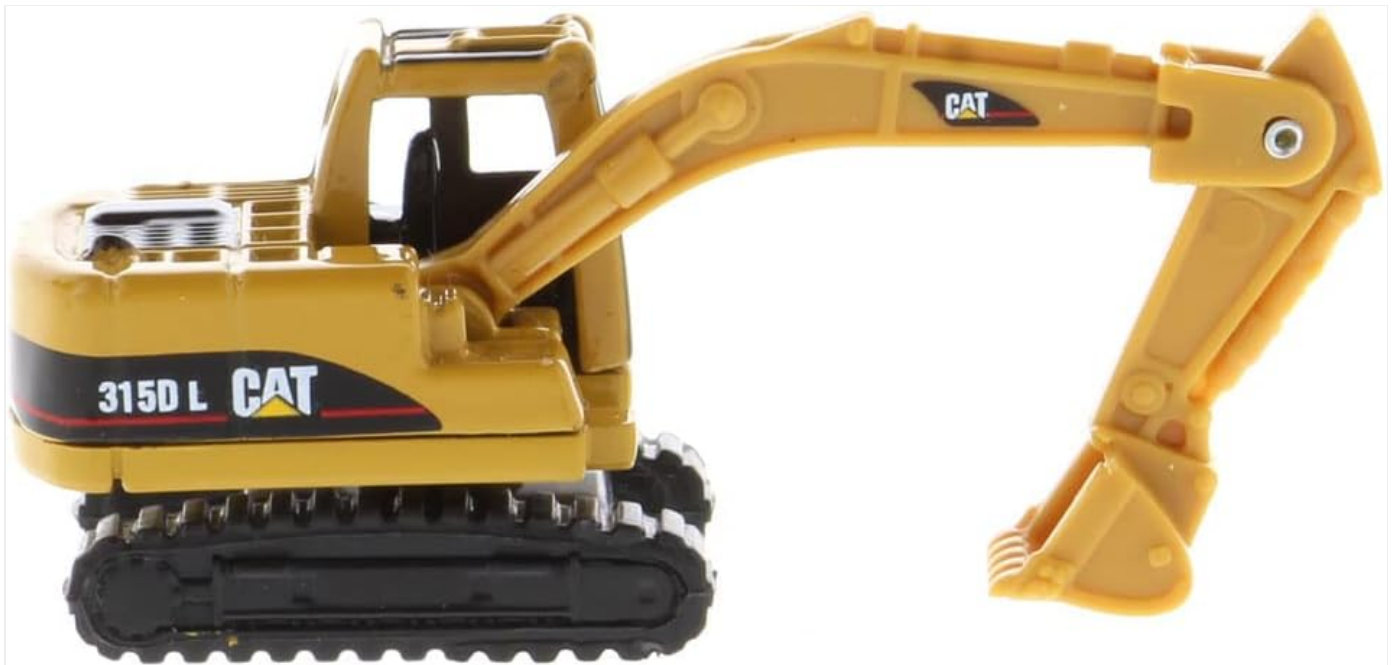
Image 2.2: Side view of the excavator model, highlighting the boom, stick, and bucket assembly.
