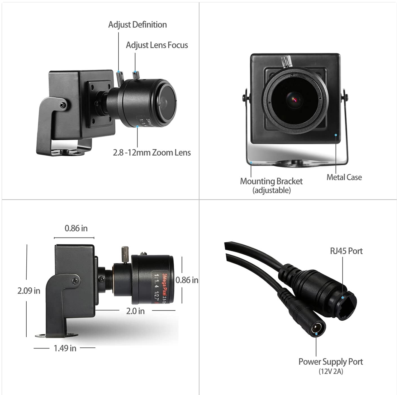
Figure 3.1: Key components of the REVOTECH I712-FHW camera. This includes the 2.8-12mm zoom lens with adjustments for definition and lens focus, a metal case, an adjustable mounting bracket, an RJ45 port for network connectivity, and a 12V 2A power supply port.
