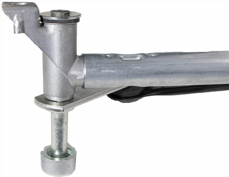
Figure 2.3: Close-up of one end of the linkage arm, showing the pivot point and connection mechanism for the wiper arm.
