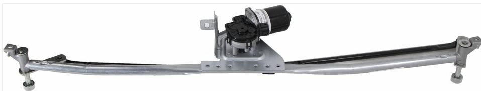
Figure 2.1: Overview of the Freightliner A22-69882-000 Windshield Wiper Motor and Linkage Assembly. This image shows the complete unit, including the motor, linkage arms, and mounting points.
