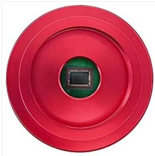
This image displays the compact, red anodized aluminum body of the ZWO ASI462MC camera, highlighting its robust construction and the central sensor area.
