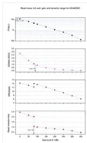
These graphs provide detailed performance data for the ASI462MC, showing the relationship between gain and read noise, full well capacity, and dynamic range, crucial for optimizing image acquisition settings.
