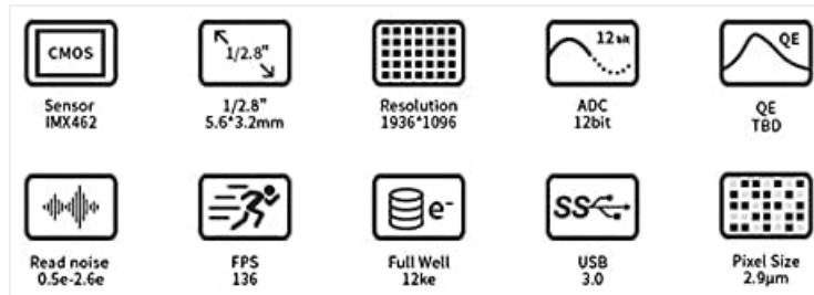
An infographic detailing the camera's core specifications: CMOS Sensor IMX462, 1/2.8" sensor size (5.6x3.2mm), 1936x1096 resolution, 12bit ADC, TBD QE, 0.5e-2.6e Read noise, 136 FPS, 12ke Full Well, USB 3.0 interface, and 2.9μm Pixel Size.
