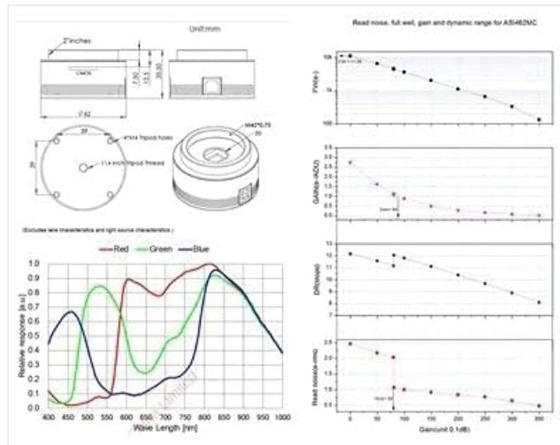
This image includes technical diagrams showing the physical dimensions of the camera and a spectral response graph indicating the camera's sensitivity across different wavelengths (red, green, blue), highlighting its infrared sensitivity.
