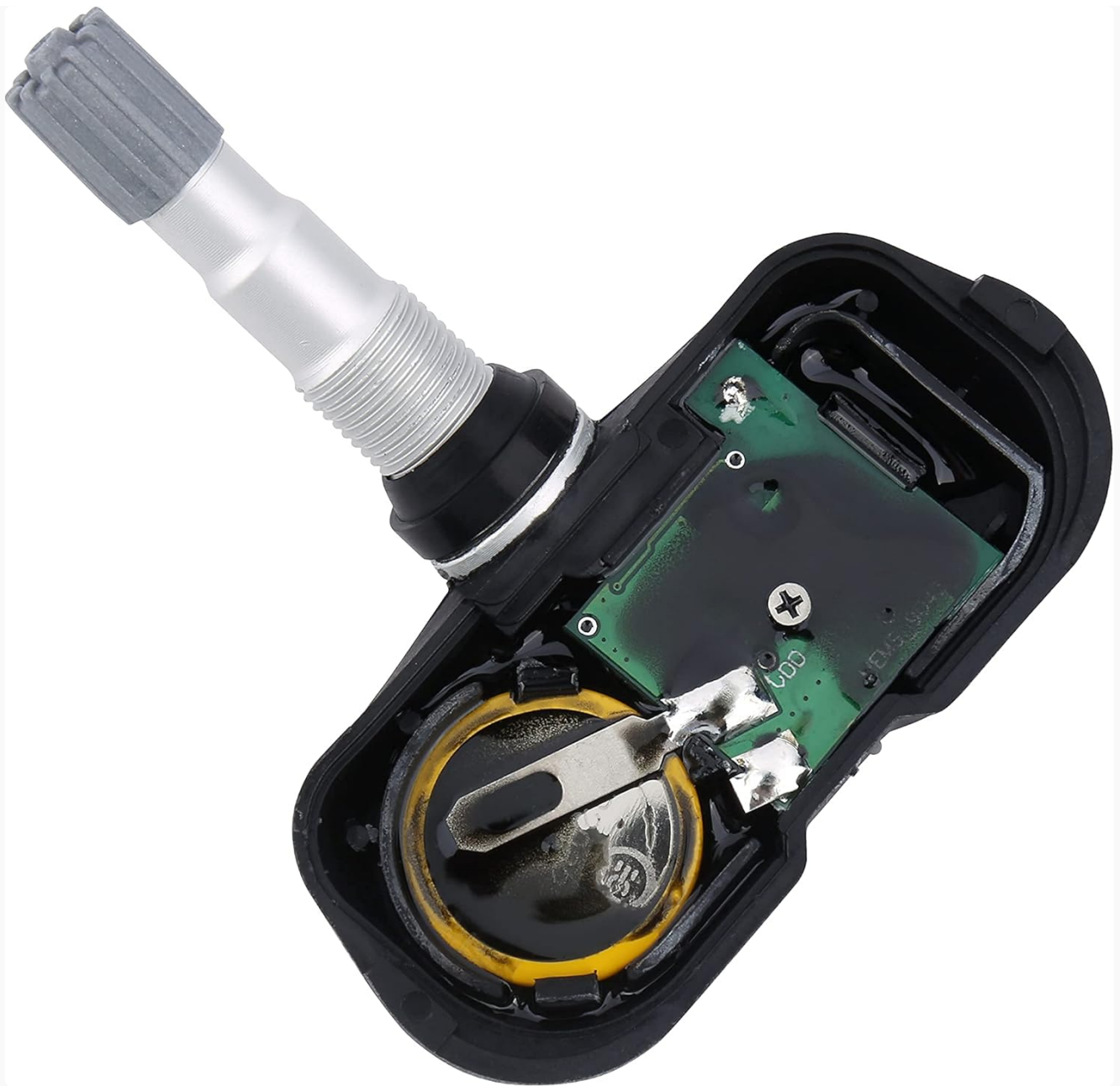
Image 6.1: Internal components of a TPMS sensor, including the battery.
