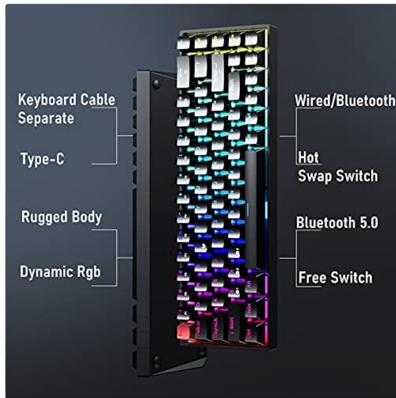
Image: Diagram illustrating the various features of the AULA F3068 keyboard, including detachable Type-C cable, rugged body, dynamic RGB, hot-swap switches, Bluetooth 5.0, and free switch capability.
