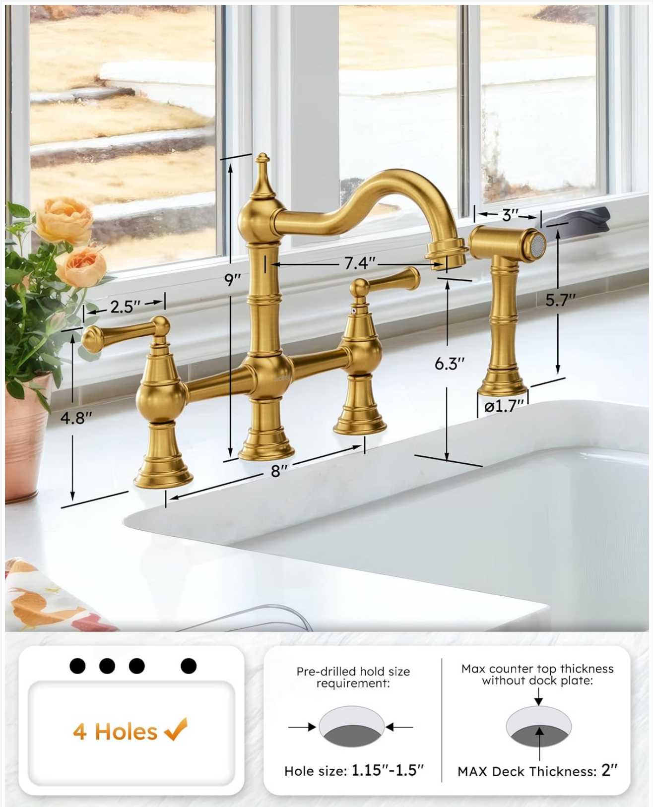
Figure 3: Faucet dimensions and 4-hole requirement.
