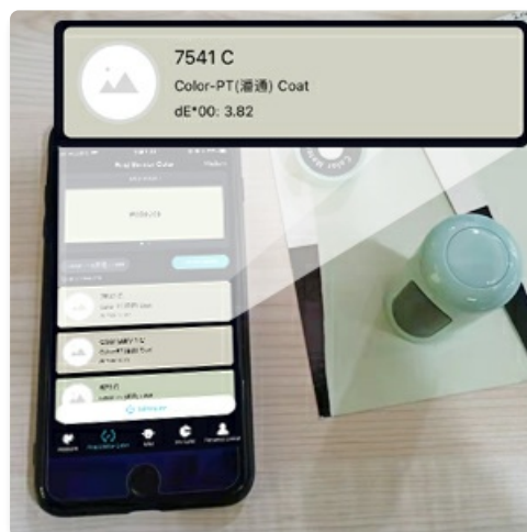
Image: Color matching functionality within the app, showing target and sample comparison.
