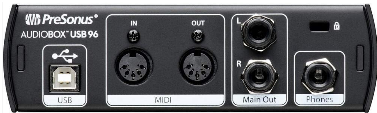
Rear view of the PreSonus AudioBox USB 96, showing the USB port, MIDI In/Out ports, Main L/R outputs, and headphone output.
