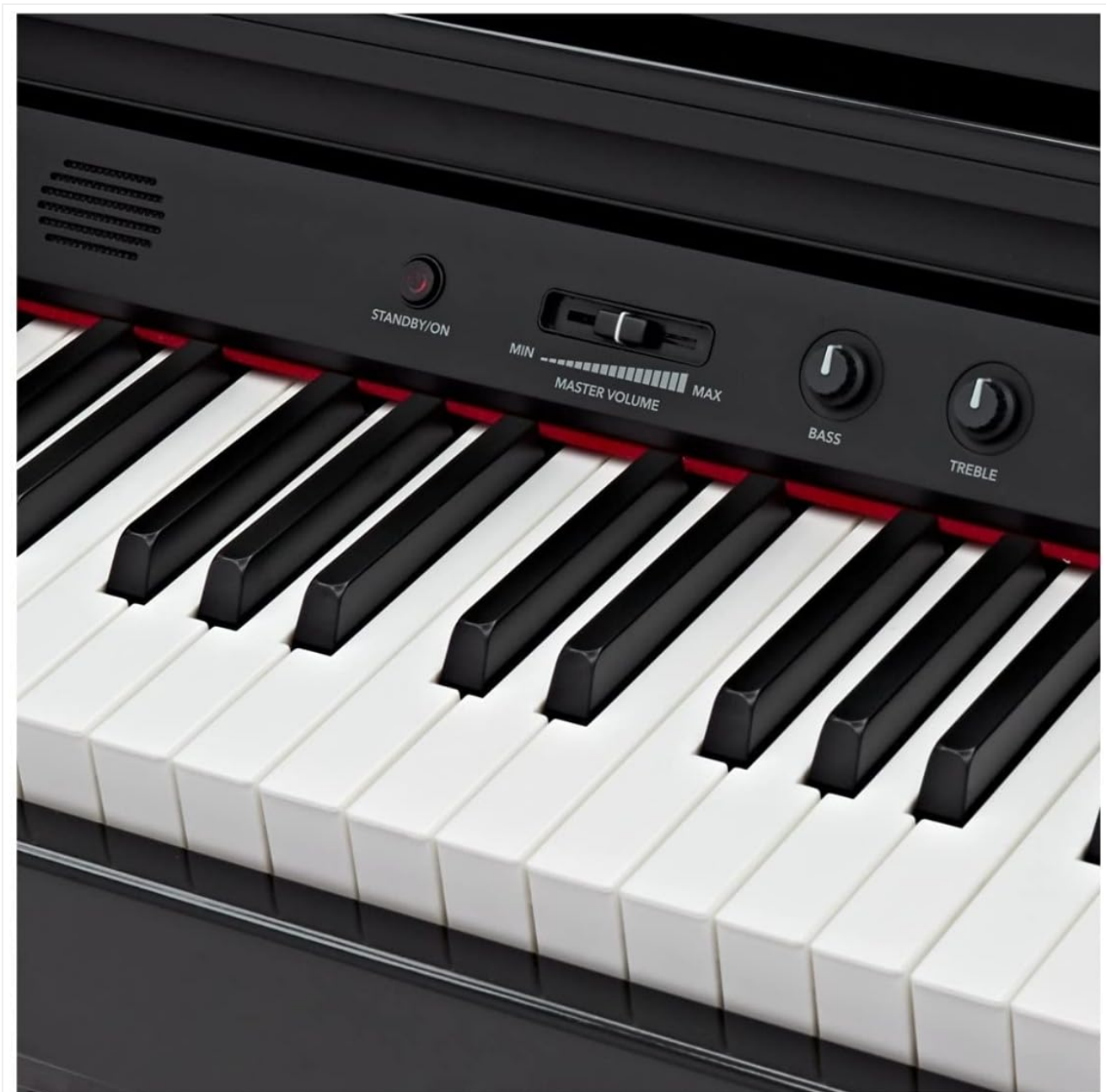
Figure 4.1: Close-up of the power, volume, bass, and treble controls.
