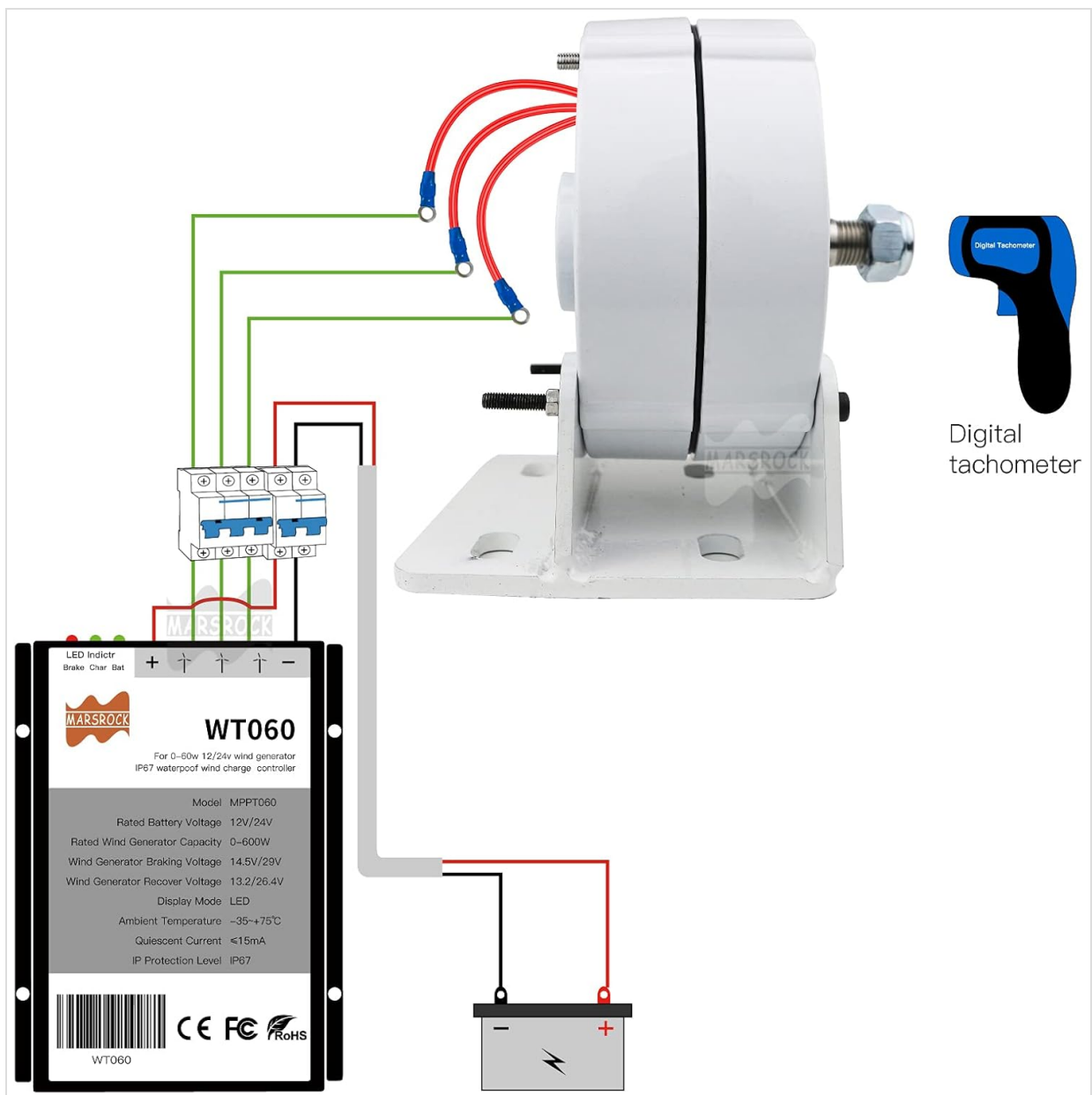
Figure 5: Example wiring diagram for the generator with a WT060 charge controller and battery. The WT060 charge controller (or similar compatible model) is crucial for converting the AC output to DC, regulating the voltage, and protecting the battery from overcharging. For more information on the WT060 controller, please refer to its dedicated manual.
