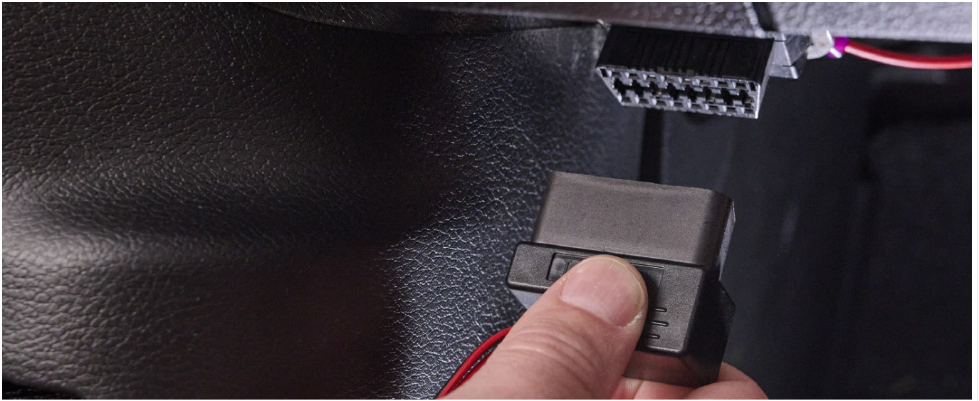
Image 2.1: Example of connecting a device to a vehicle's power source, often found near the fuse box or OBD-II port.
